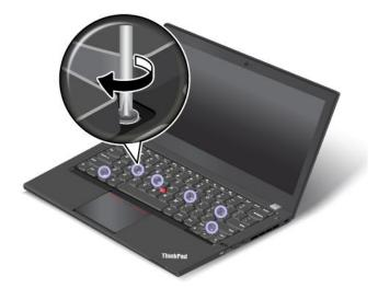
5. Slide the keyboard frame backward by 2.5 mm (0.1 inch) with the keyboard multi-tool. Hide the latches of the keyboard frame under the keyboard bezel by pushing the latches with your finger as shown.
